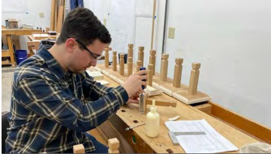
Sean Dye, one of the shop's newest co-workers, is putting felt on stoppers. These stoppers will go in a rank of wooden pipes and help create the tone as well as tune the pipe.
